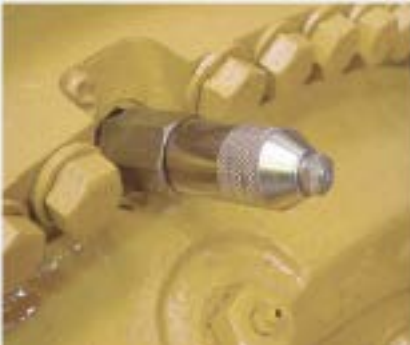
Birrana™ brake wear gauge fitted
